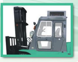
Other optional items include the windshield and wiper as well as airconditioning and heating units. These ergonomic aspects promise an overall comfortable, convenient and safe working space for truck operators.
